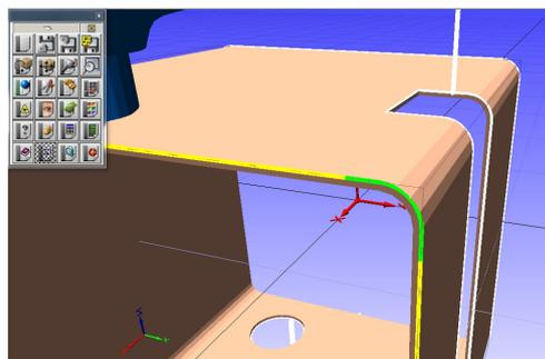
Through extensive checks, the program ensures an exact cutting path and actively warns the user about any possible collisions between the laser head and the elements to be machined.
