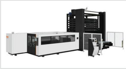
CMC is a compact, 10 pallet stoker for OPTIPLEX 3015 CO2 and Fiber configurations. It features a 1" thick material capacity, 2,200 pound plate capacity and optional sorting station.
